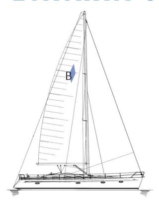
Length overall 50'6" Length hull 49'2" Length waterline 44'2" Beam 14'9" 6′1″ Draft standard Draft (deep lead option) 6'11" Displacement 27,720 lbs. Ballast 9,240 lbs. Water tank 200 gal. (appx.) Fuel tank 85 gal. (appx.) 1,405 sq. ft. (appx.) Mainsail & genoa Ht. of mast above waterline 68'
